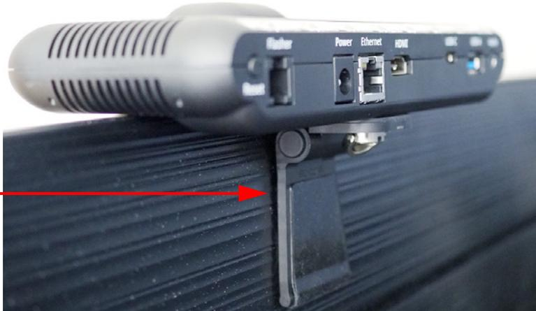
Bracket adjusted for thick display panel
