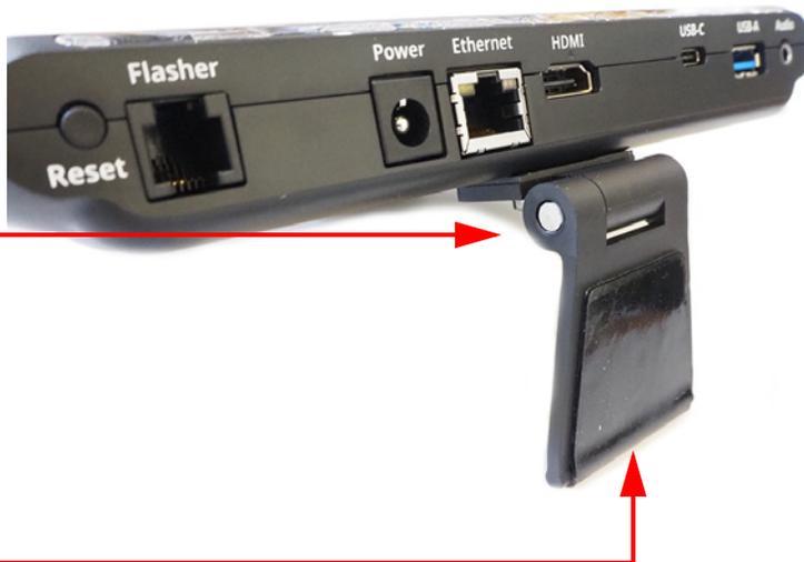
Notice the clear plastic sheet that is covering the adhesive surface on the lower part of the Camera Bracket. You will usually **not** need to remove this sheet to mount the Lumina videophone to your display. Simply leave the sheet in place on the bracket.
