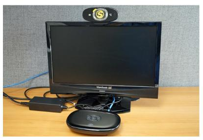
Figure 5 — nVP2 Main Unit, power supply and camera on video display
