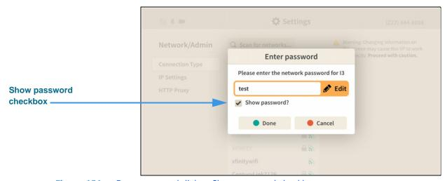
**Figure 151** — Enter password dialog, Show password checkbox
