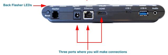
**Note:** The USB-C port on the Lumina Main Unit does **not** support Thunderbolt displays (e.g., only the HDMI port can be connected to a external HDTV or display). Do **not** connect anything to the USB-C port because it is reserved for future use.
