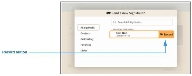
Figure 94 — Record button revealed
