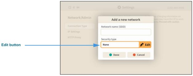
Figure 153 — Add a new network screen, Security type Edit button
